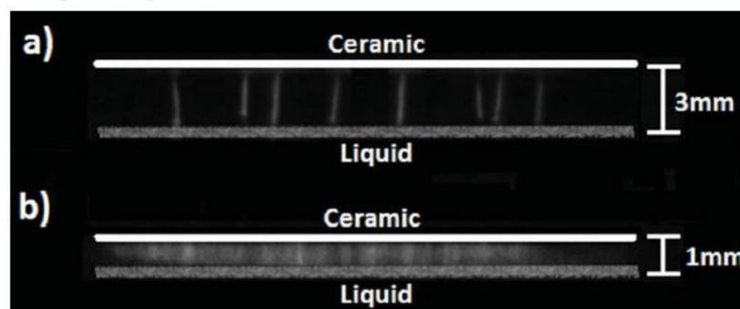
FIG. 2: iCCD pictures of the sinusoidal (a) and nanosecond-pulsed (b) DBD plasma. Exposure time 210  $\mu s$  (a) and 1  $\mu s$  (b)
