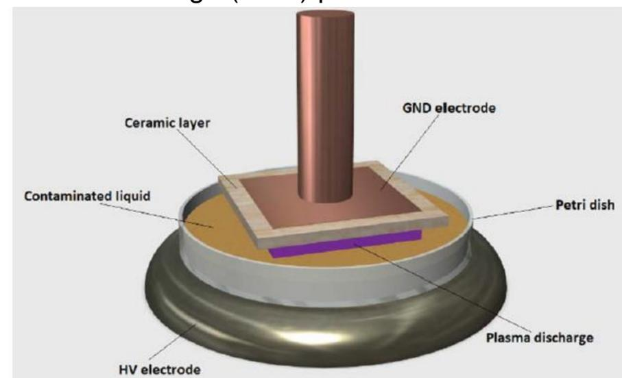
FIG. 1: Schematic of the DBD device
